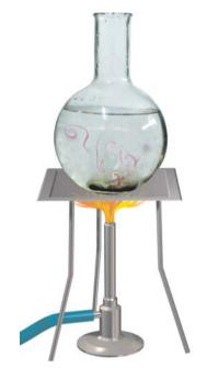
Fig. 4.9 Convection of heat in water
