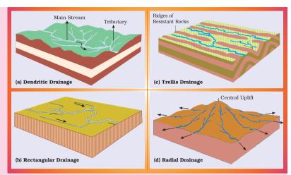
terrain. The radial pattern develops when streams flow in different directions from a central peak or dome like structure.
