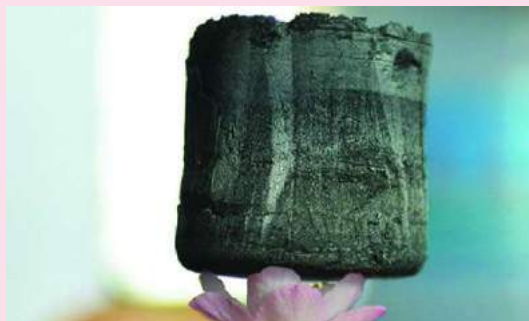
A piece of graphene aerogel - weighing only 0.16 milligrams per cubic centimeter - is placed on a flower.
