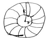
Width of Embank w = 7m Inner radius r = radius of well = 7m Outer radius of Embank R = r + w= 7 + 7 = 14 m Area of base of Embank =  $\pi R^2 - \pi r^2$ =  $\pi (R^2 - r^2)$ =  $\pi [(14)^2 - (7)^2]$ =  $\frac{22}{7} [7^2 (2^2 - 1)]$ =  $\frac{22}{7} [7^2 \times 3]$ =  $\frac{22}{7} \times 7^2 \times 3$ =  $22 \times 7 \times 3 m^2$
